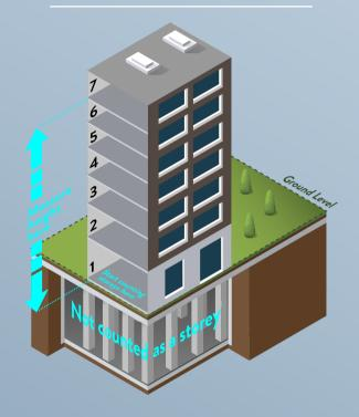
For Diagram A, **storeys are counted from the first above-ground level**, and height is measured to the top storey's floor surface. This structure has 7 storeys.
