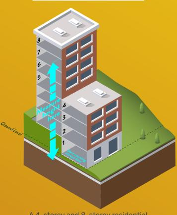
A 4-storey and 8-storey residential tower are connected by a party wall on sloped ground. This **combined structure** is **considered** 8 **storeys**.
