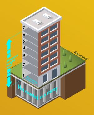
Storeys should be counted from the **first level above ground**, and height measured from ground level to the top storey's floor surface. In Diagram A, the building is 7 storeys high according to the Regulations.
