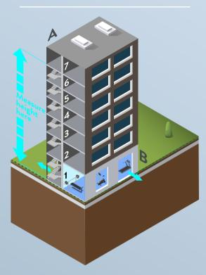
Diagram C shows a 7-storey residential tower (A) with a ground-floor gym (B) having separate access. Tower A is a higher-risk building with 7 storeys.
