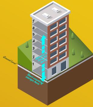
For buildings on sloped ground, ground level is the **lowest point touching the structure**. Height is measured from this lowest ground level to the top, and storeys are counted starting above ground level.
