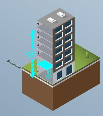
Diagram F shows a 7-storey tower with a gallery floor exceeding 50% of the area of the storey above. The gallery is counted as a storey, making the building 7 storeys.
