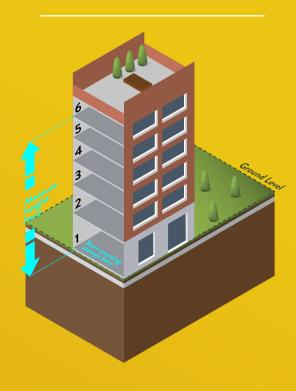
Measure height to the top storey's **floor surface**, excluding rooftop gardens. In buildings where the top level is machinery or plant rooms, height is measured to the floor of the storey below.
