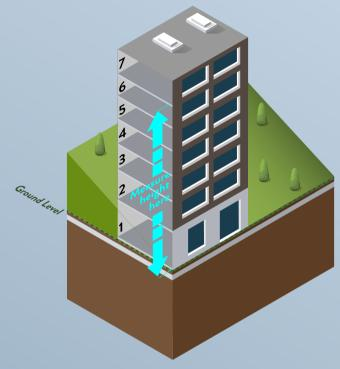
For buildings on uneven ground, height is measured from the **lowest ground level touching the structure**, and storeys are counted starting above ground. The structure in Diagram B has 7 storeys.
