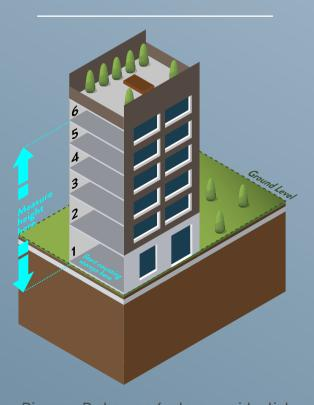
Diagram D shows a 6-storey residential tower with a rooftop garden. Height is measured to the top storey's floor surface, excluding the garden. The structure has 6 storeys.
