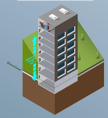
Diagram E shows a 7-storey tower on sloped ground with a rooftop plant room. Height is measured to the top storey's floor (not the plant room). The building is 7 storeys and higher-risk as it has two or more residential units.
