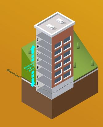
For a 7-storey residential tower on **sloped ground** with a rooftop plant room, **height is measured from ground level to the top residential storey**, not including the plant room.
